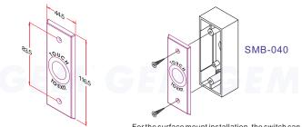
For the surface mount installation, the switch can be mounted with SMB-040 black plastic casing or SMB-Unit: mm 040Mfor stainless steel housing.
